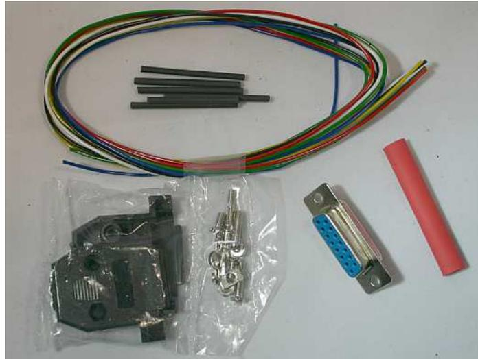
Strip a few millimeters of the six colored wires and solder them to the female DB015 connector. The solder cups are numbered from left to right: 1 ... 8. You use only the top row, the bottom row has only 7 cups. From left (1) to right (6) the wire colors are black, red, green, blue, yellow and white.
