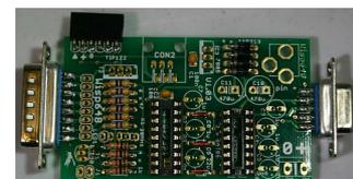
Place and solder the LED. The longer wire must be put in the hole in the middle of the silk 'symbol' for the LED. In other words: insert the longer wire in the hole nearest to the DB15 connector. Trim the wires.
