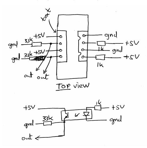
Without current through the LED side the voltage on the 'out' terminal is less than 0.1 Volt. With the 1k resistor approximately 5 mA flows through the LED and the voltage on the out terminal rises to 3 Volt.
