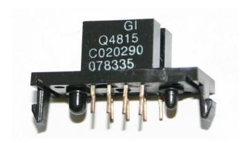
This interruptor has eight pins which match a DIP 8 grid. It contains two LEDs (I assume IR, because I don't see any light) and two foto transistors (or maybe foto diodes). I tested the part with the circuit shown below.
